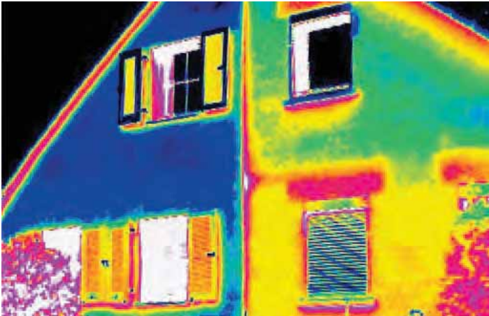
Image produced with a Thermographic Camera.
